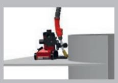
/ Welding fillet welds on convex components
