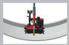
/ Welding butt welds on concave components
