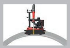
/ Welding butt welds on convex components
