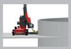
/ Welding fillet welds on convex components
