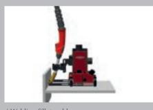
/ Welding fillet welds on horizontal components
